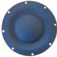
The TU diaphragm has a rod connection only at the air side and an easy to clean liquid surface. This means no ink or paint residue will accumulate behind bolts, center disks etc. which prevents color contamination. Temperature Range: 0°C to 85°C with a short peak load up till max 100°C
